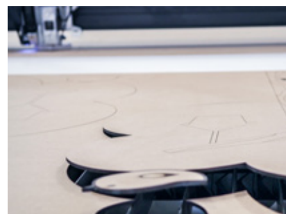
Laser cutting of MDF furniture. Within seconds from design to reality.
