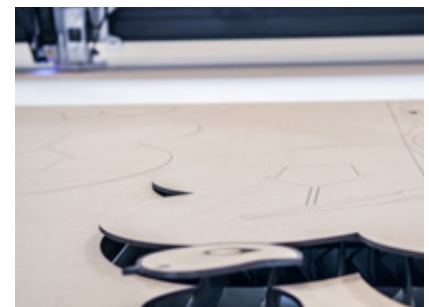
Laser cutting of MDF furniture. Within seconds from design to reality.
