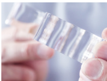
Flame-polished result. Cut up to 40mm acrylic.
